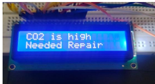
Fig. 10: Close-up of LCD displaying “CO 2 is high / Needed Repair” threshold-violation alert, confirming correct ASCII generation, 8-bit parallel data transfer, and HD44780 enable/RS timing at 100 MHz.
