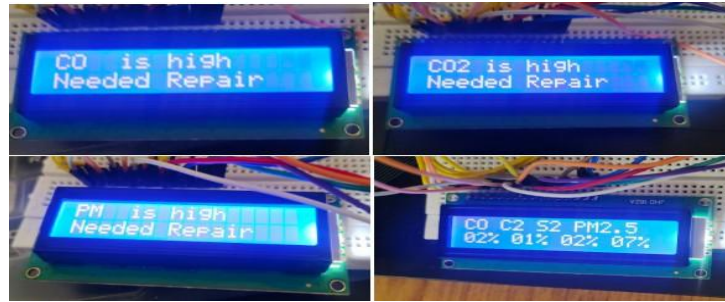
Fig. 9: LCD output states: (a) CO alert — “CO is high / Needed Repair”; (b) CO 2 alert — “CO 2 is high / Needed Repair”; (c) PM 2.5 alert — “PM is high / Needed Repair”; (d) Normal operation — “CO 02% C2 01% / S2 02% PM 2.5 07%”. All states confirmed in hardware.
