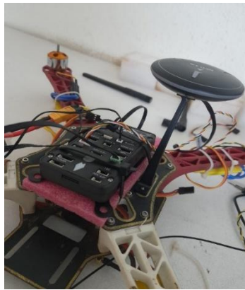
Fig 1 : Quadcopter with Neo3 GPS and Pixhawk flight controller
