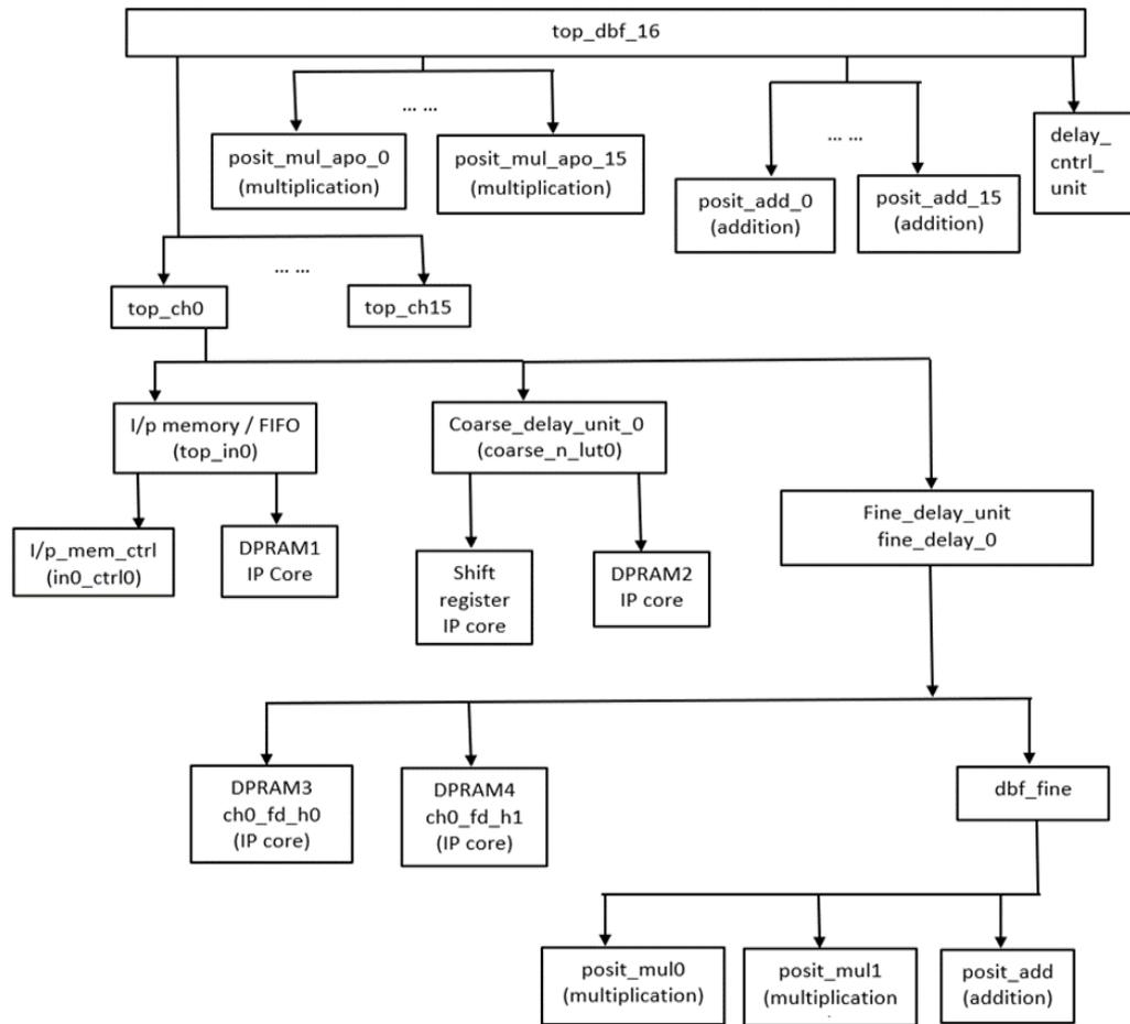
Fig. 6. Design flow diagram of posit arithmetic-based digital beamformer.
