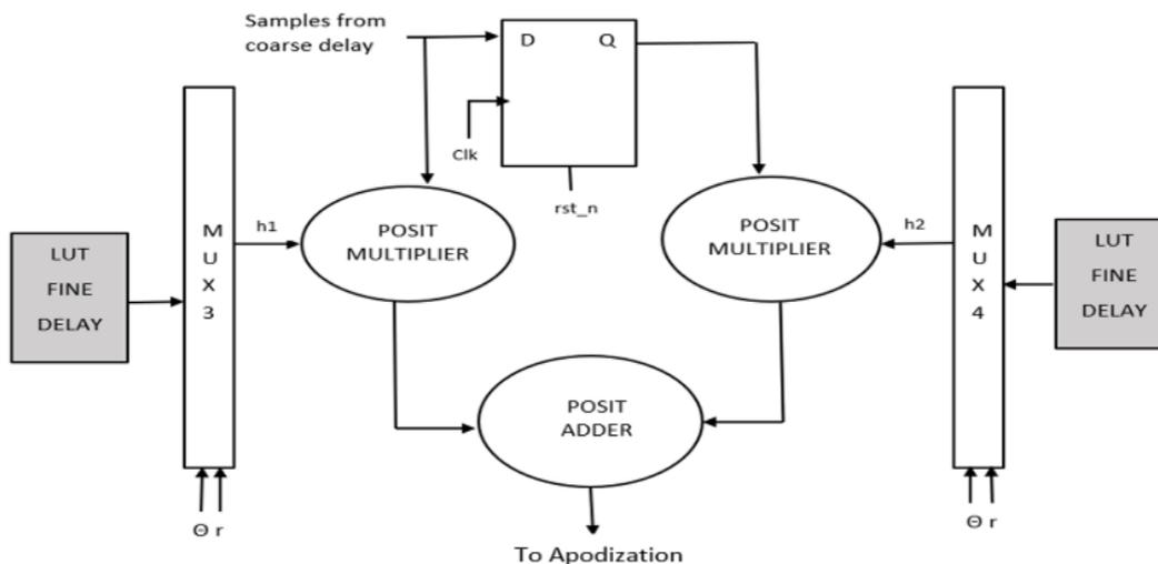
Fig. 4. Block diagram of Fine delay unit.
