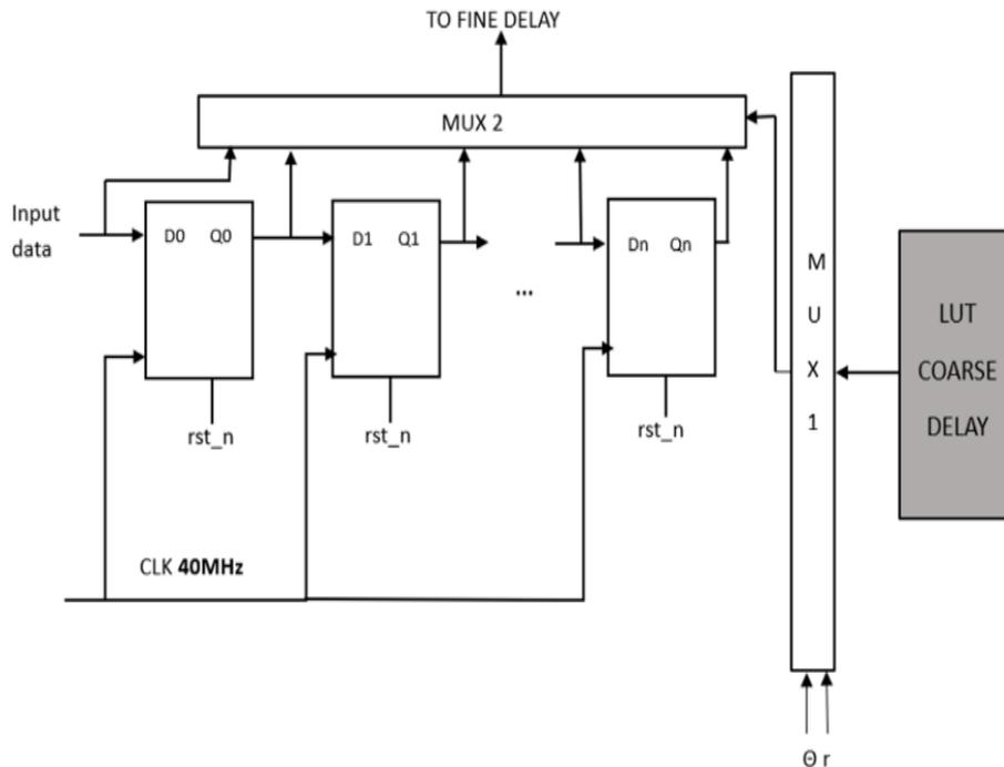
Fig. 3. Block diagram of Coarse delay unit.
