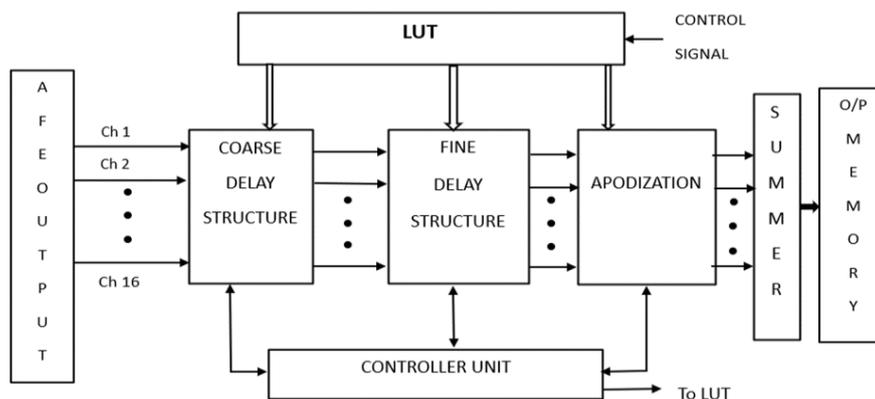
Fig. 2. Block diagram of delay and sum beamformer showing delay elements.
