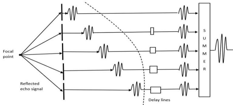
Fig. 1. Block diagram of linear phased array beamformer.
