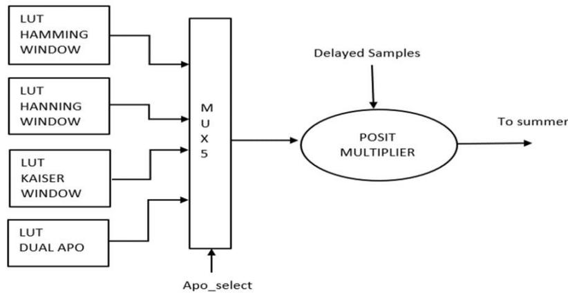
Fig. 5. Block diagram of Apodization unit.
