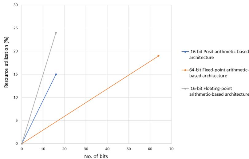
Fig. 8. Resource utilization comparison.
