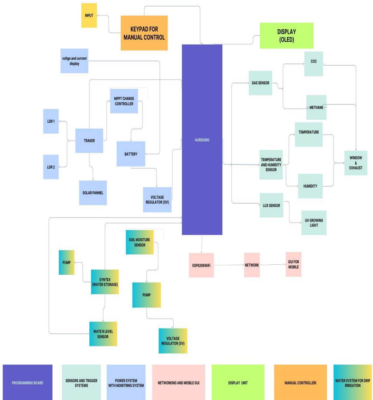
Fig. 1. Block Diagram of the Smart Green House, smart Irrigation system and battery Monitoring System .
