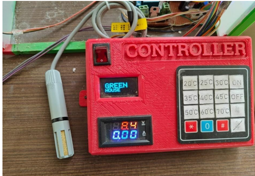
Fig. 3. Setup of keypad with interfaced with oled
