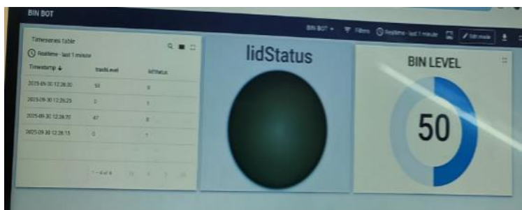
Fig. 8. Dashboard displaying bin level and lid closed status
