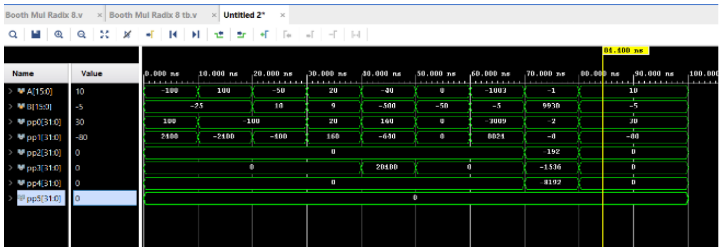
Fig. 3 Simulation waveform of Radix-8 Booth multiplier showing signed partial product generation and accumulation.
